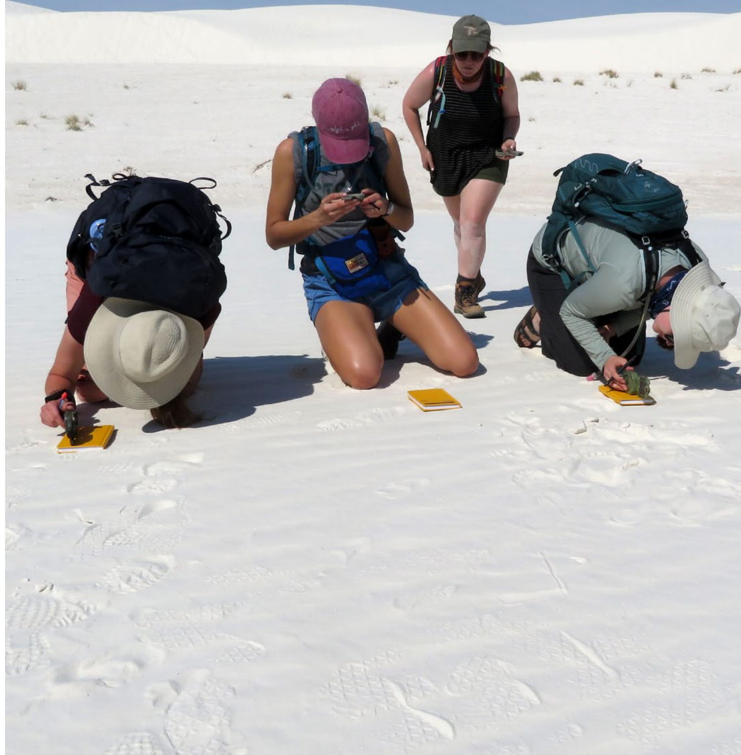
PRACTICING MEASURING STRIKE AND DIP ON THE LEE FACE OF A DUNE AT WHITE SANDS NATIONAL PARK.
