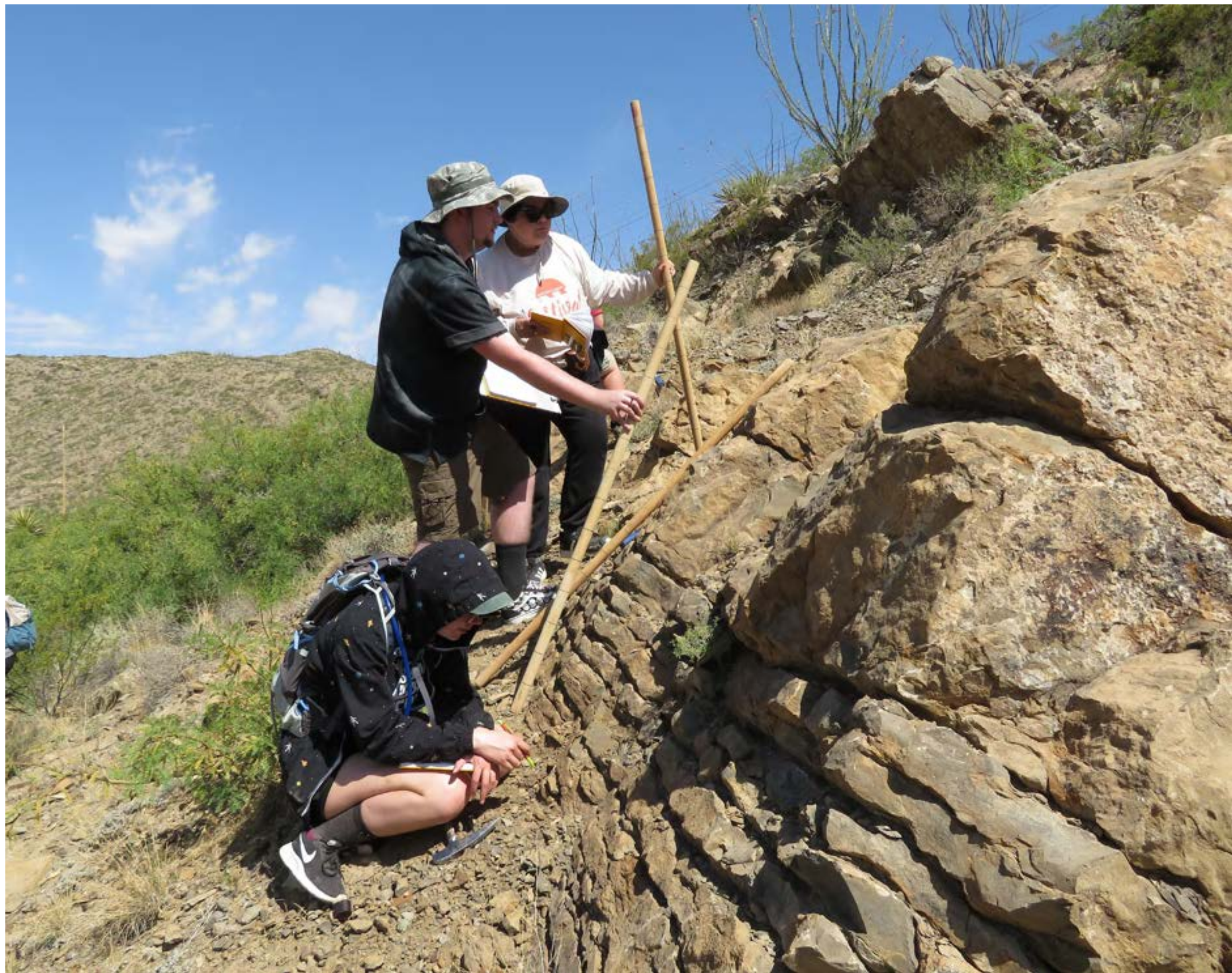
The students discuss the correct orientation to hold their Jacob staves while measuring section.
