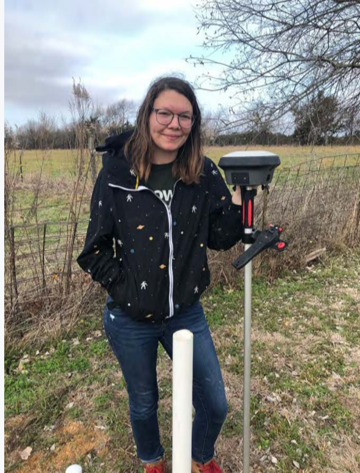
Taylor Watson surveying piezometers on World Hunger Relief Inc property as part of her BS thesis research.
