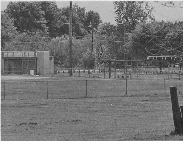
Fig. 33. A common use of flood plain land is for public parks. Cyclone fences around these parks not only accumulate debris and retard flood flow, but are capable of withstanding more force and will not likely be flattened by flood waters.
