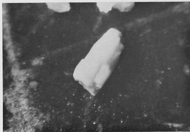
Fig. 51. (Locality 41) Photomicrograph (x140) of medium-sized grain of kaolin pseudomorphs after potassium feldspar.
