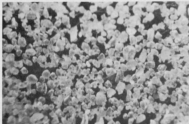
Fig. 24. Sub-angular, well sorted very fine sand and coarse silt from the intertidal facies. Georges Creek Member. Locality 22. (x 31.5)
