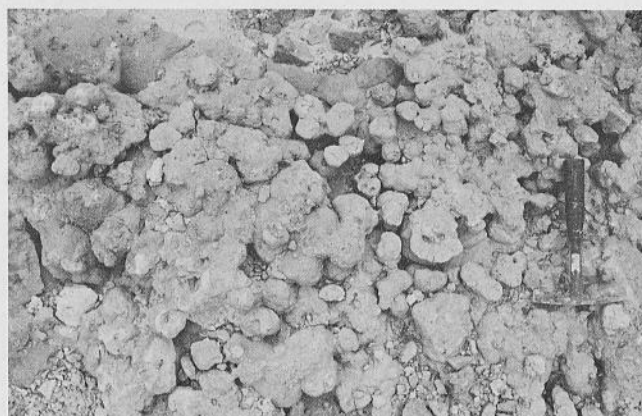
Fig. 33. Caliche horizon. Note the nodular character of the bed. Georges Creek Member. Locality 15.
