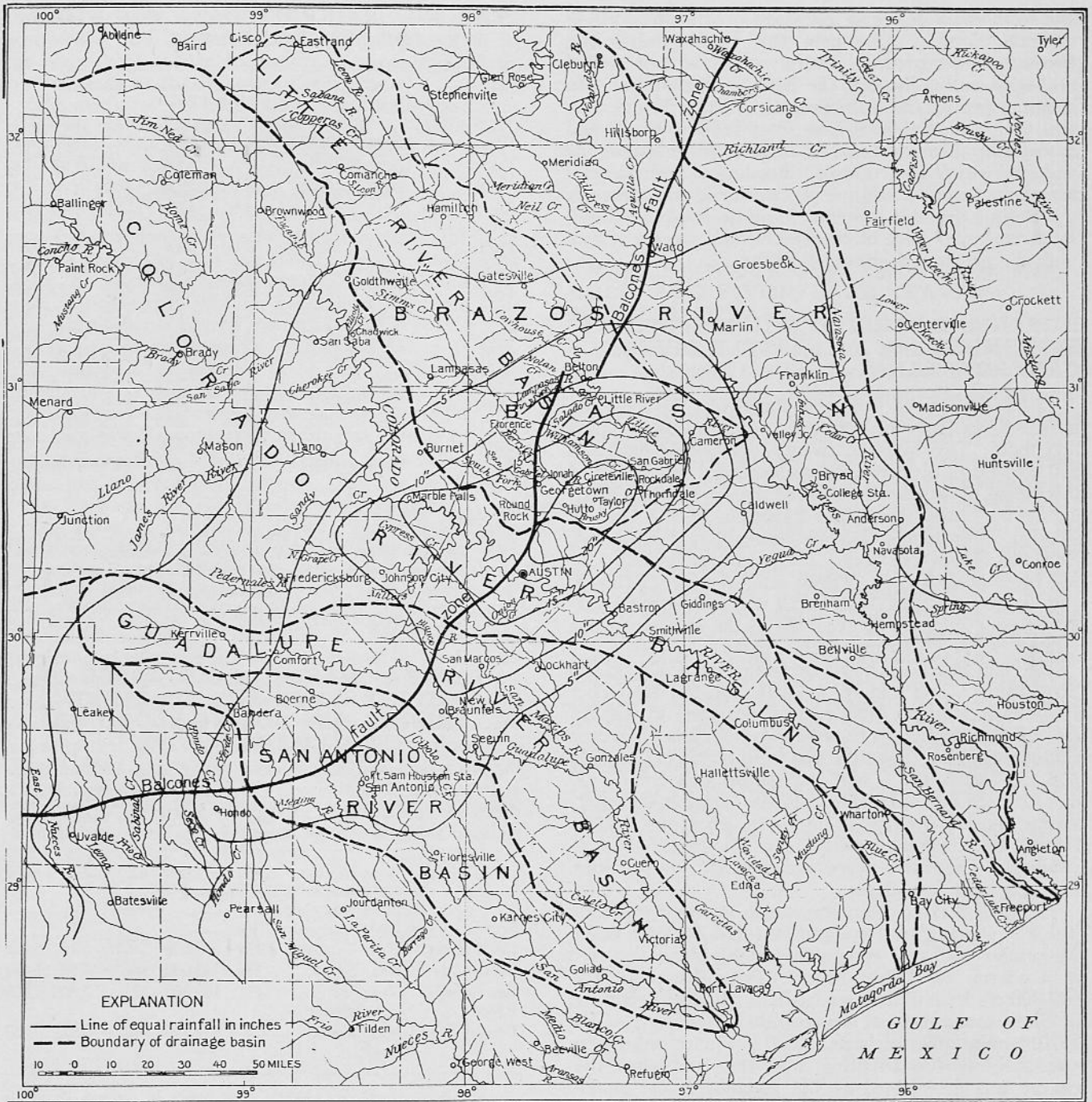
Fig. 6. Map of central Texas showing drainage basins and total rainfall September 7-11, 1921. From Ellsworth, 1923, U.S. Geological Survey Water-Supply Paper 488, Plate I.
