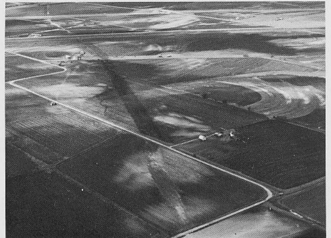
Fig. 18. Aerial photograph of the corridor about five miles south of Waxahachie, Texas (gas pipeline transects area from upper left to lower center). Whiter areas are thinner Eddy-Stephen and Brackett soils. Gray areas are Austin series soils. Black areas are Houston Black soils.
