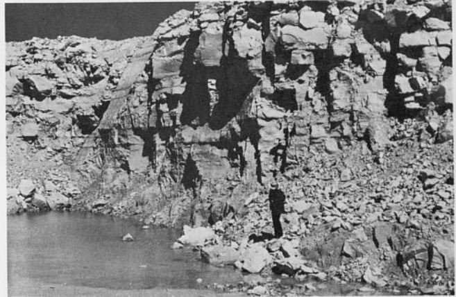
Fig. 5. Massive, dense "upper" Austin Chalk in quarry south-east of Waxahachie (Loc. 6). Note dominant joint patterns and spacing (two to five feet). Marl layers are deeply recessed and thin (five to 24 inches).
