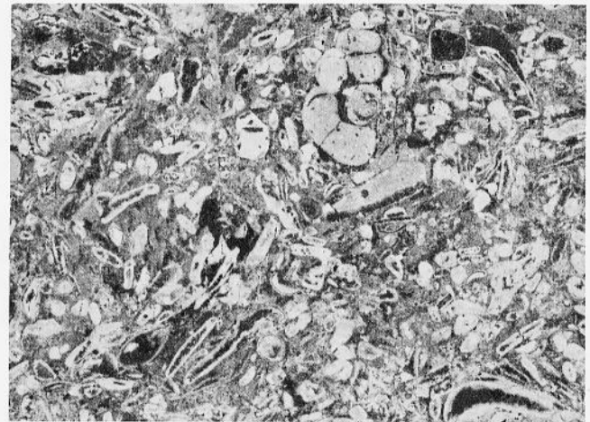
Fig. 10. Thin section (X 25). Poorly washed, moderately packed to packed, fossiliferous fecal intrasparite with mollusk fragments and encrusting blue-green algae. Negative print. Locality 27, bed 26.
