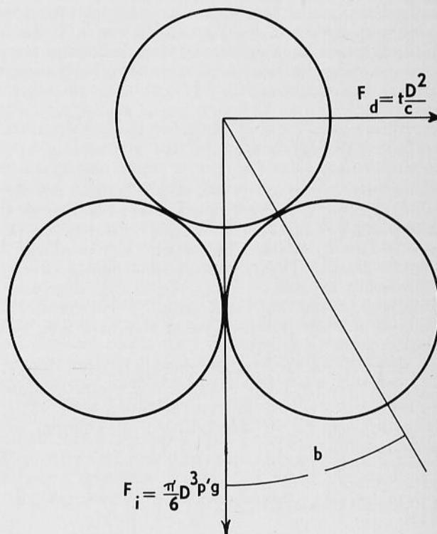
Fig. 28. Forces acting on a bedload particle.
