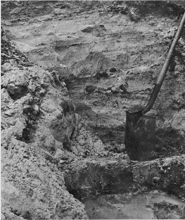
Fig. 6. Point bar stratification, Brazos County (Locality 2). Lower Unit, moderately sorted medium sand overlain by six inches of red clay. Upper Unit, poorly sorted cross-bedded gravelly sand with clay balls overlain by coarse gravel in a clay matrix.
