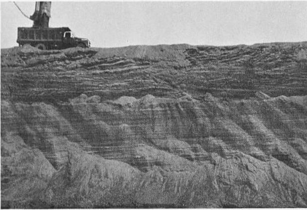
Fig. 10. Point bar sequence, Robertson County (Locality 4). Lower unit, large sets of trough cross-stratified sandy gravel and sandy gravel foresets. Contact zone, thin discontinuous slightly oxidized medium sand. Upper unit, organic rich black clay. The thick clay unit represents back-swamp and oxbow deposition.
