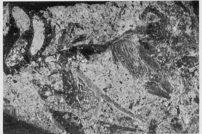
B. Sample 25, Locality 2-4. Calcite crystals filling voids. Dark areas are limonite inclusions. This limonite is secondary, resulting from oxidation of primary pyrite inclusions (x 15). This picture is a negative image.
