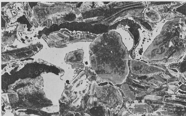
Fig. 27. Limestone petrography of washover beds of elongate reefs. Sample 21, Locality 5-8. Elongate reef sample composed of biomicrite. Included within this sample are inclusions of limonite, altered from primary pyrite (x 25).
