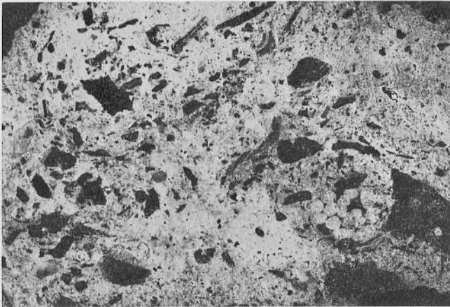
A. Sample 1, Locality 2-8. Shell fragments with a sparry calcite rim. Solution has occurred and spar is filling the voids (x 15). This picture is a negative image.
