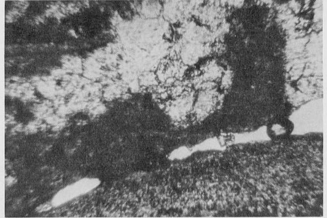
B. Sample 4, Locality 1-1. Elongate reef biomicrite shows calcite and voids.
