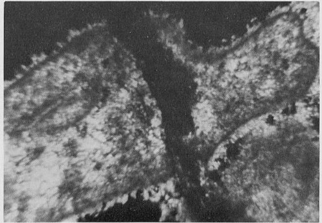
B. Sample 21, Locality 1-3. Calcite fills the voids in the sample. Limonite is dominant throughout the slide as dark inclusions. Note the large fecal pellet in the left center of the photograph (x 50).
