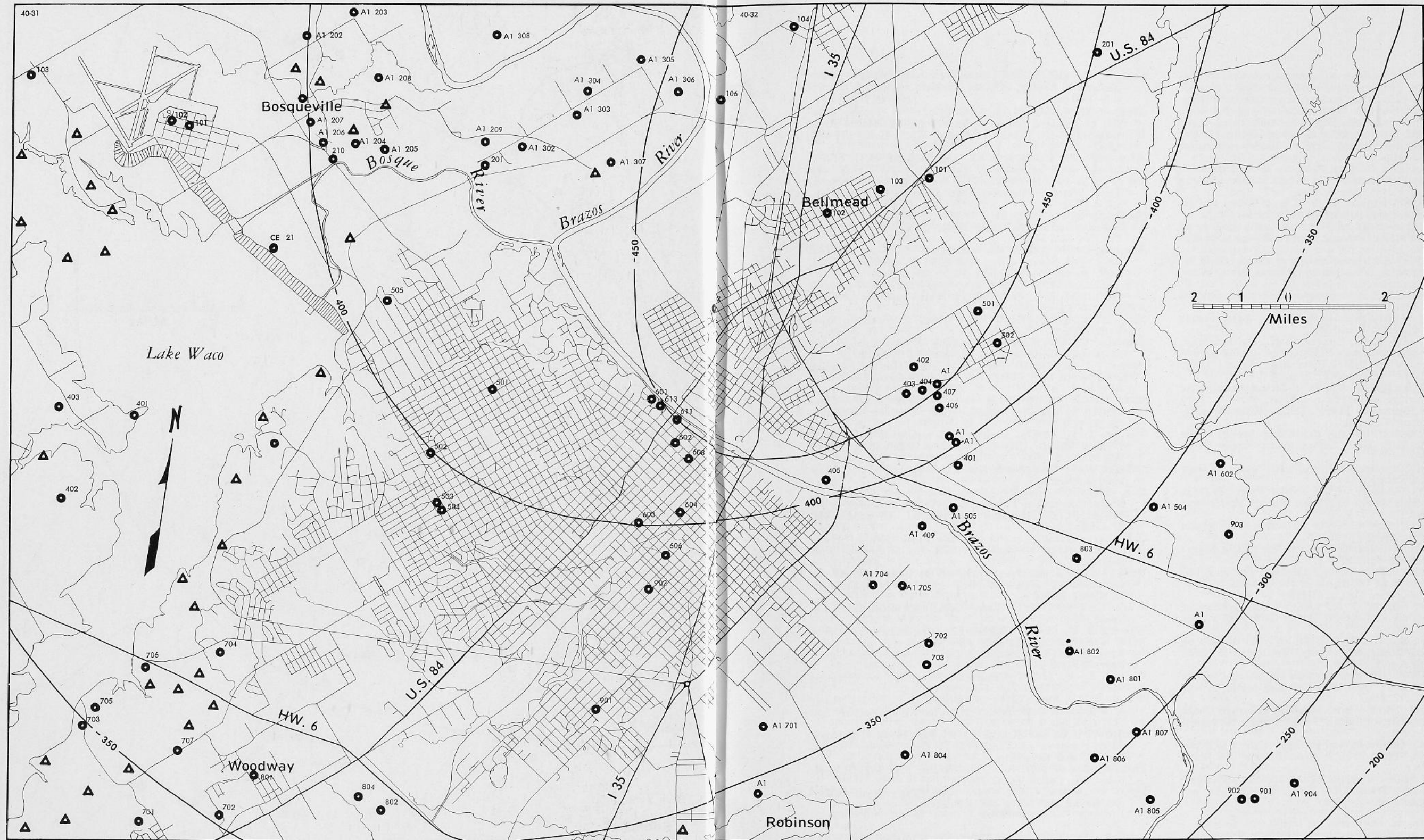
Fig. 33. Water-level decline in wells, Trinity aquifer, 1900-1967. Data from TWDB unpub. Trinity aquifer study—Klent, Perkins, and Alvarez, 1975.
