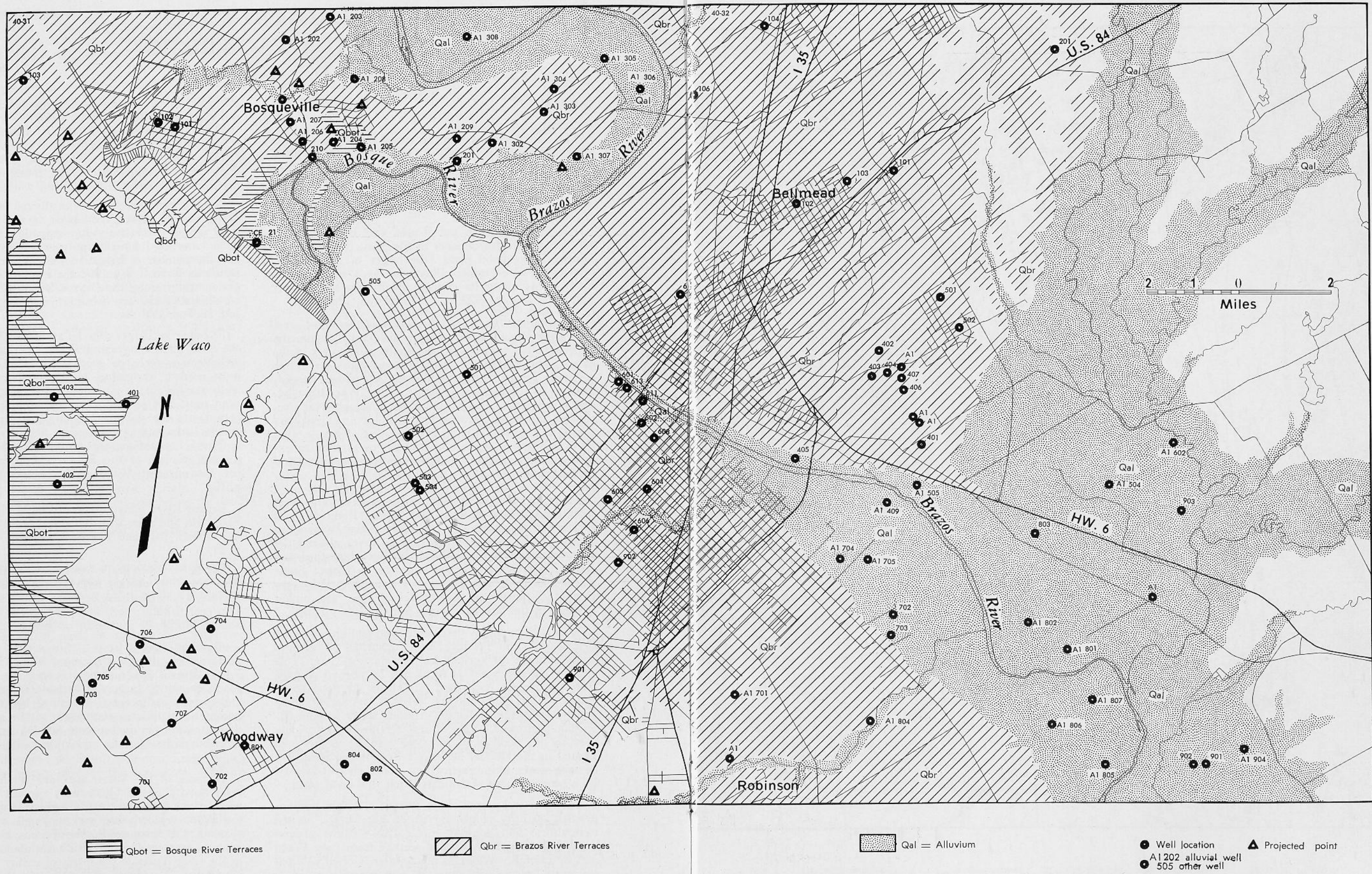
Fig. 9. Surface geologic map showing extent of terrace and flood-plain alluvium. Terrace and alluvial wells are indicated by solid dots.
