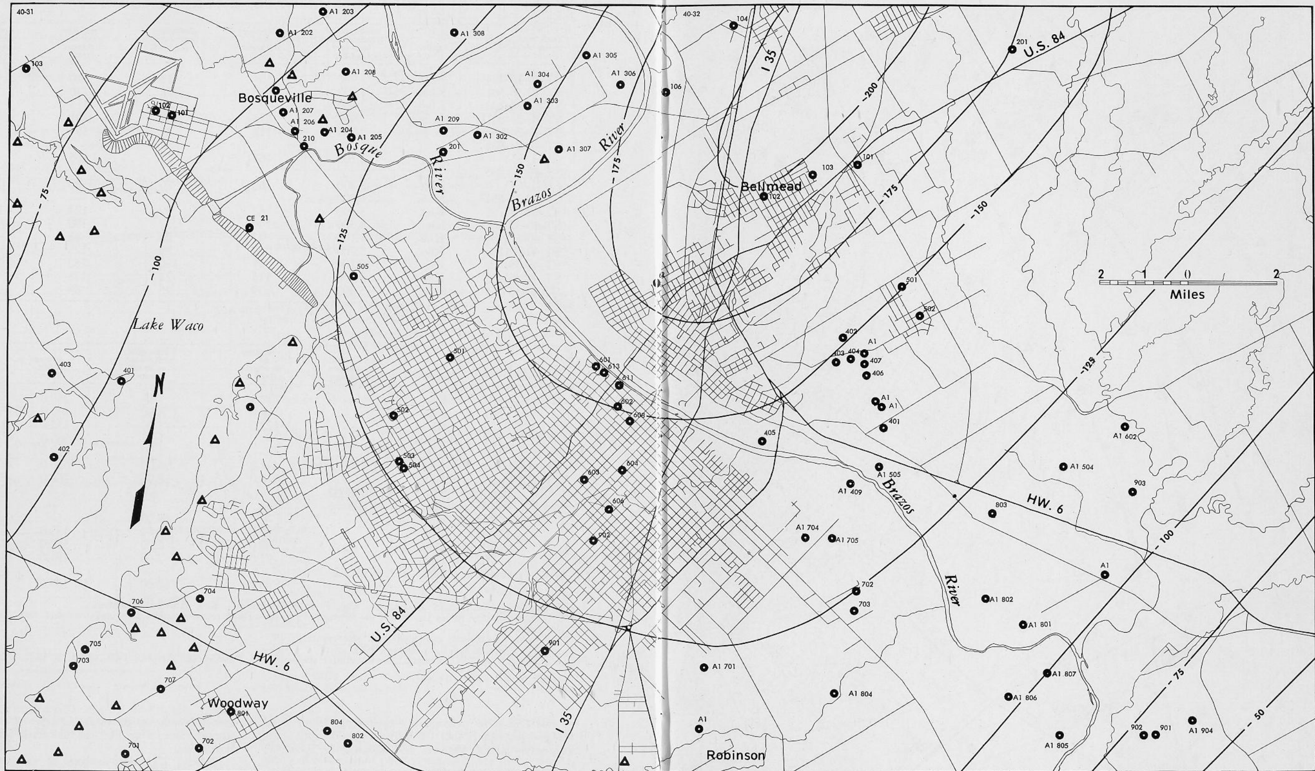
Fig. 24. Projected water-level decline, Hensel Formation, 1975. Data from TWDB unpub. Trinity aquifer study—Klent, Perkins, and Alvarez, 1975.
