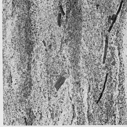
Fig. F. (154-B-44, unit 16) Foraminifera bio-micrite. Acetate peel. Large recrystallized calcite fragments of Inoceramus are common; dark-gray arcs contain clay. (x2)
